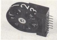
Model H5220 is a TTL-compatible, magnetic-wheel, 12-V unit designed to be driven by a 5445/7445 BCD-to-decimal driver. It has an op temp range of —55 to 95°C, meets MIL-STD-202 environmental requirements, may be mounted on 0.295" centers, and is available with pins for direct PC board mounting or with lead wires for harnessing. Novatronics of Canada Ltd, PO Box 610, Stratford, Ontario, Canada.
