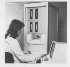
model. The MB7464 is based on a minicomputer with 48-k store and includes a fast printer and a visual display unit (VDU) with keyboard. The test program and diagnostic data are produced on a single floppy disc and may be read directly by a Membrain MB2420 or MB-2460 test system. Optionally, the test program may be punched on paper tape for use with any Membrain automatic test system. The price quoted (station plus software) is f.o.b. Ferndown, U.K. Stand No. 19321 Circle No. 449
