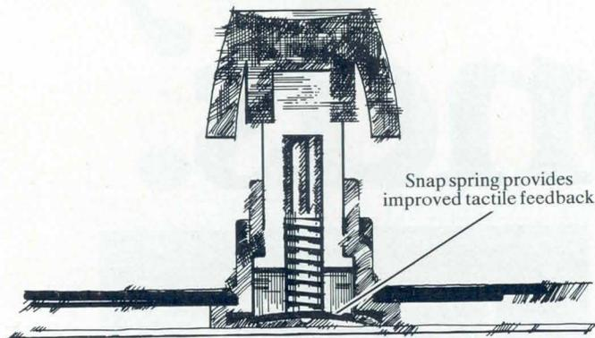
And, the actuator module for the full-travel membrane keyboards helps achieve new levels of tactile feedback and operator satisfaction.
