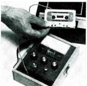
Tension monitor model M-100 measures dynamic tape tension between drive capstan and two tape packs within digital and audio cassette decks. Monitor uses special cassette, instrumented internally with a strain gage containing 150 ft of tape. Information Terminals Inc., Terra Bella Ave., Mt. View, Calif. [366]
