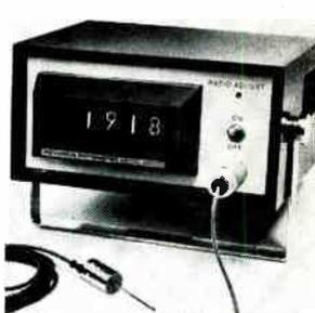
Displacement measuring system acts as ratiometer, providing system accuracy to  $\pm 0.1\%$  + one digit. Other types of dc-dc linear variable differential transformers with displacement ranges of  $\pm 0.02$  ft to  $\pm 5.0$  ft are available. Price starts at \$510. Pickering and Co., 101 Sunnyside Blvd., Plainview, N.Y. [368]
