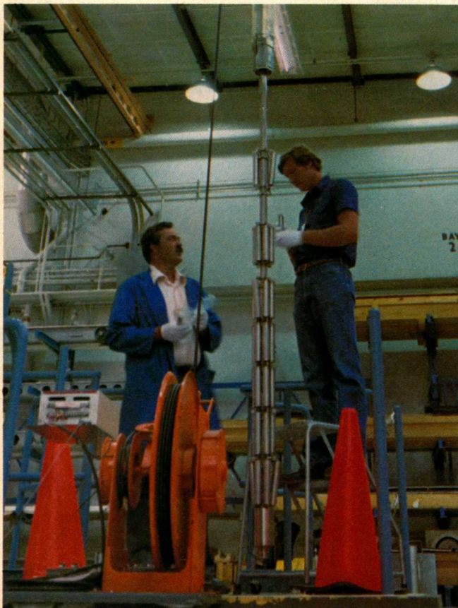
Small canisters of metal specimens undergo fast, breeder-like stress tests at Westinghouse Hanford Fast Flux Test Facility.
