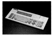
The Hi-Tek keyboard line offers custom layout, full encoded models suited for the simplest or the most sophisticated systems. The 100 million cycle mechanical keyswitch can be employed in the DIN standard, low profile layout. Membrane keyswitches are also available for custom applications in low cost systems.
