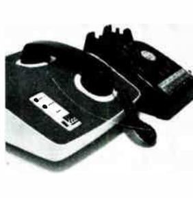
Acoustic coupler model DD 103 AC converts EIA or TTY signals to standard frequency shift keyed signals for transmission over phones. Bit serial data is transmitted in a form compatible with 103A data set. Features include half/full duplex circuitry, coherent switching, accurate carrier detect. Digi-Data Corp., 4315 Baltimore Ave., Bladensburg, Md. 20710 [403]
