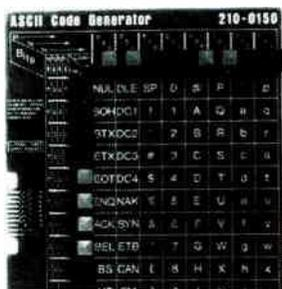
Code generator produces all 128 characters of the 7-bit ASCII code without a full-size keyboard. It is wired for positive logic, with a bounce-free, TTL-compatible output, and requires a 5-Vdc power supply. Light-emitting diodes display bit levels. Generator requires no special skill to operate. Price is \$98. Mechanical Enterprises Inc., 5249 Duke St., Alexandria, Va. 22304 [402]
