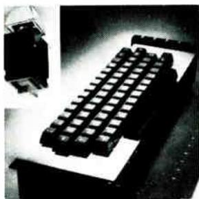
Modular solid state keyboard FS 300 eliminates encoding electronics and electrical contacts, and reduces component count. A ferrite key switch with one moving part develops the code. Power consumption is as low as 50 mA at 5 V for a full 88-key board. Logic level outputs are DTL- and TTL-compatible. Port Electronics Products, 133 Brimbal Ave., Beverly, Mass. 01915. [401]
