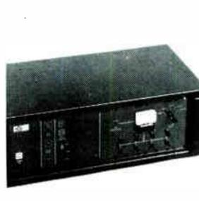
Modem with a symbolic status display is insensitive to virtually all bit patterns. The 4,800-b/s modem, designated the model 248A, is macromodular in construction, and the multicolored display instantly indicates the condition of the modem. Packaging is stand-alone or for cabinets. Information Exchange Systems Inc., 3312 Gorham Ave., Minneapolis, Minn. [407]
