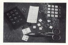
Keyboard features removable clear cap key tops permitting easy exchange of key legends to match programming needs. Conductive elastomer sealed switches are standard with X-Y matrix, X-common, and Y-common; no interface circuitry is required. Form A with single common also is available. Keys have 0.075" travel and are on 0.650" centers. Tactile snap is optional. Both 12- and 16-key versions are available. Flex-Key Corp, 18 Sargent St, Gloucester, MA 01930.
