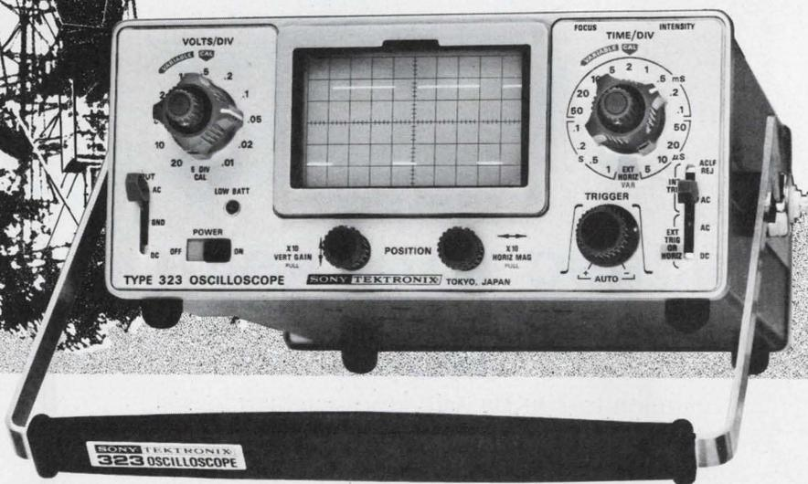
The **SONY/TEKTRONIX Type 323** Portable Oscilloscope weighs 7 lbs, is 4 1/4 inches high, 8 1/2 inches wide and 10 5/8 inches deep. It operates from self-contained batteries for up to 7 hours. With this compact, lightweight instrument, a user may move from one remote application to another without concern for power connections.
