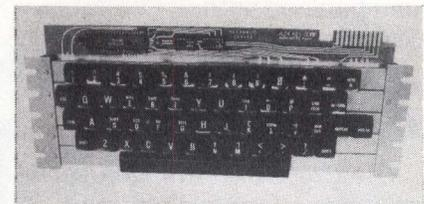
FlexMatic CEK-33, a 53-key, quad mode, USASII-coded ASR-33 keyboard, is available with either 2- or n-key rollover. Using a conductive elastomer switching technique, the unit has a full 0.18" keytravel, 0.05" overtravel, truncated 2-shot molded keycaps, and solid-state ROM encoding, and is fully compatible with TTL and MOS logic arrays. Switches are completely sealed and environment proof and are rated for 50 million operations min. **Flex-Key Corp**, 18 Sargent St, Gloucester, MA 01930.
