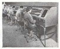
DEXON INC., 3517 Raleigh, Minneapolis 16, Minn., is producing a fully government-approved line of modularly connected Primaire climate control cabinets capable of providing dust, temperature and humidity control in a start-to-finish assembly line setup. This includes instrumentation such as ultrasonic cleaning, flushing, filtering, baking, balancing, sealing, curing and inspection. (347)
