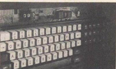
Full function programmable keyboard uses a single-chip 8-bit microprocessor that incorporates ROM and RAM, as well as an erasable p/ROM, which enables complete software control of all key functions. Microprocessor also permits automatic repeats, multiple programming of a single board, program changes in the field, serial and/or parallel I/O, and n-key rollover (3-key rollover is std). Reed keyswitches are low profile, measuring 1.03125" (0.793
