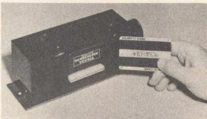
Series LC-31 Gameloader™ conveniently loads programs for home/hobby computers. Programming/data storage media holding 1k 8-bit bytes is the company's 4-stripe Kilobyte Card.™ An enclosed strobe controlled PC/LED/shaft encoder provides data accuracy independent of head speed. A 2-channel R/W type head provides recording densities of 420 bits/in (165/cm) on the card, with typ ISO/ANSI-std 2.81" (7.14-cm) track length. Char load time is 5k bytes/min. Read speed is 3.1"
