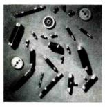
Thin film resistors are designed for microwave applications. Film is deposited by pyrolytic carbon process. Substrate is aluminum or beryllium oxide. Temperature coefficient of resistance is 250 ppm/°C, and standard resistance tolerance is 1%. Midwest Microwave Inc., 3800 Packard Rd., Ann Arbor, Mich. [345]
