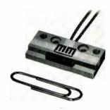
Ferrous-operated proximity reed switch, model 26-23, for industrial control is highly stable unit with 2-millisecond response. Actuation range is .075 to 0.150 in. in .025-in. steps. Initial contact resistance at 25 ma is 0.5 ohm max for laboratory grade. McClintock Matrixes Inc., Woodbury, Conn. [348]
