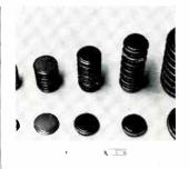
Sealed, non-gassing mercuric oxide cadmium batteries have shelf life of 5-10 years and operational temperature capability of -65° to 164° F. They are available in five capacities from 500 ma/hr to 12 a/hr. Voltage can be any multiple of 0.9 v. Elca Battery Co., 1140 W. Evelyn Ave., Sunnyvale, Calif. [342]
