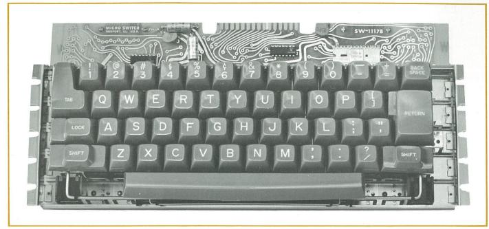
The 51SW12-1 keyboard is ideally suited to word processing and phototypesetting applications, especially where high speed alphanumeric data entry is performed by operators previously trained as touch typists. Every effort has been made to duplicate the operation of an office typewriter—to reduce operator training. This includes key array, buttons, key operating force, N-Key rollover interlock and more.
