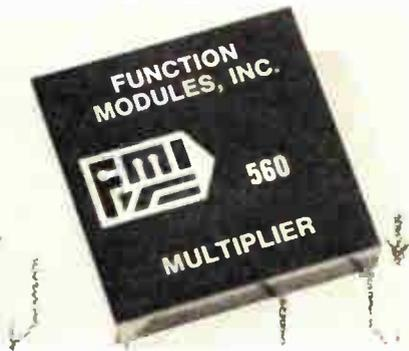
Irvine, Calif., is introducing a four-quadrant transconductance multiplier that boasts a maximum full-scale accuracy of within  $\pm 0.1\%$  and that costs only \$139 in quantities of 1 to 9. The accuracy figure applies to operation in any quadrant and over the full input voltage range of  $\pm 10$  volts. Moreover, since all linearity, gain, and offset errors are accounted for in the accuracy specification, the unit's nonlinearity is held to a mere  $\pm 0.04\%$ .
