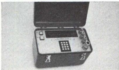
Portable display terminal has std uc ASCII keyboard with optional numeric pad. Char size is 0.28 x 0.20" in 5 x 7 dot matrix. Display is neon-orange plasma with 256 char in eight 32-char lines on 3.3 x 8.7" screen (128 char in four lines on 0.8 x 7.1" screen optional). Operating modes are full- or half-duplex or local. Block mode is optional. Transmission code is 7-bit ASCII plus 1-bit parity (switch-selectable even, odd, 1, or 0). Transmission speeds are 110
