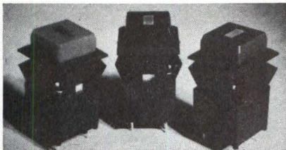
Series offers seven different background button colors with red, yellow, and green LEDs. Centered in a 1/2" button, the 0.100 x 0.250" window displays the LED at a 150-deg viewing angle. Added reliability is provided by stationary LEDs that remain fixed during switch operation. Switch also features 2M cycles at logic level loads using bifurcated contacts and is practical where low contact resistance, bounce, or noise prevail—both audible and electrical.
