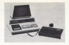
The desktop, steel enclosed keyboard connects to the computer through a plug-in interface card. Once installed, it is usable on all existing software. Sharing the computer's internal keyboard interface allows the two keyboards to be used interchangeably; thus, the remote unit can be used for normal data entry and the built-in unit for numerics or graphics.
