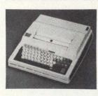
Silent 700<sup>™</sup> model 765 portable memory terminal and model 763 send-receive terminal come with 20k bytes of nonvolatile TBM 0103 bubble memory storage, expandable to 80k bytes in 20k-byte increments. Units can access any indexed record in memory in <15 ms; if the data location in 765 memory is not known (not in-
