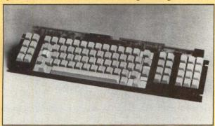
A sense amplifier detects changes in capacitance. It incorporates an ANY-KEY-DOWN output that is monitored when other keyboard electronics are applying a pulse drive. Linear or pad tactile feel is available with a positive stop. Full 0.15" (3.81-mm) nom travel is standard. Operating force is 2 oz; 21/2 oz is an option. Sculptured and/or stepped spherical keycaps are also available. Cherry Electrical Products Corp, 3600 Sunset Ave, Waukegan, IL 60087. See at Booth P7035
